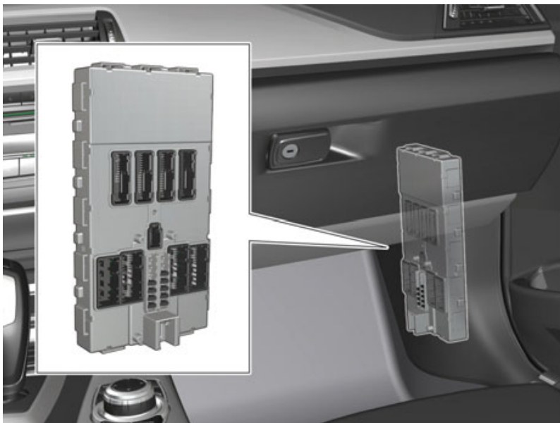
F30 FEM installation location
